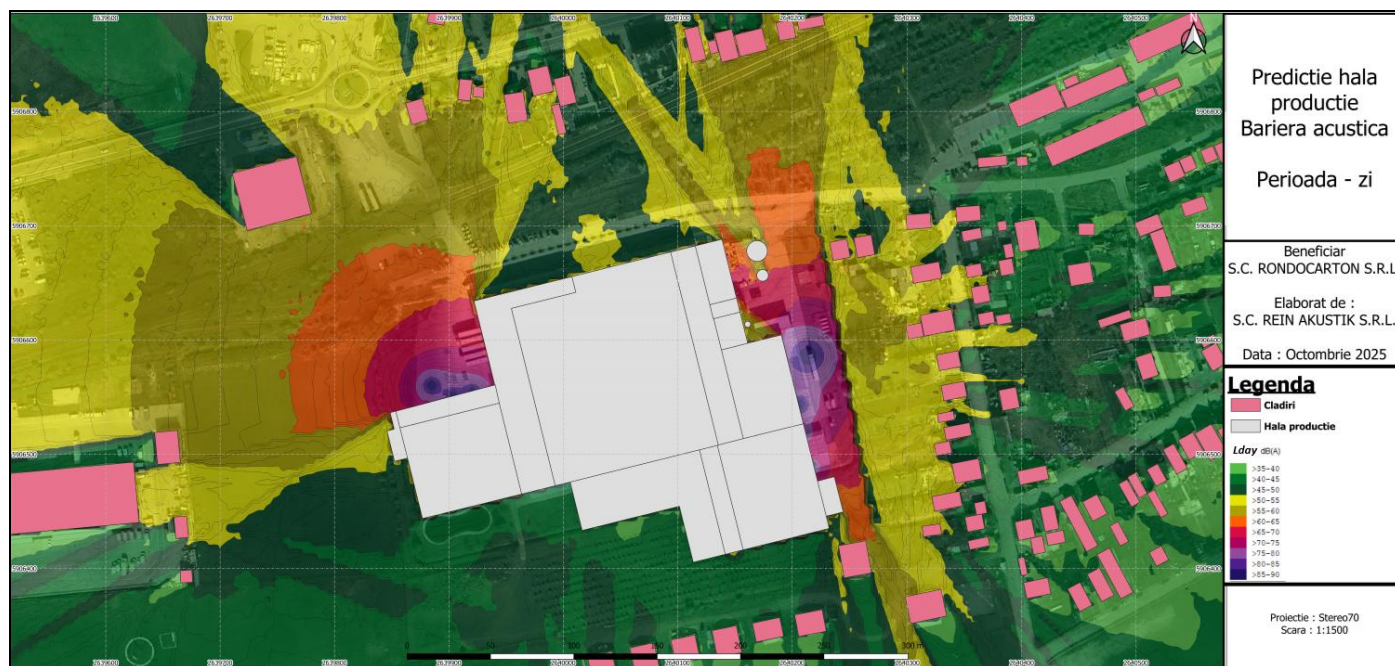
Figure 36. Noise levels map during the day period, with acoustic barrier L_{day} [dBA]
