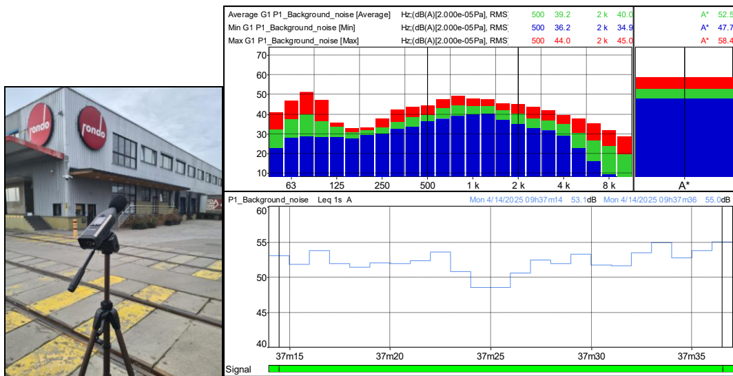
Figure 6. Measuring point P1 – Entrance gate 1 P1_gate_factory background noise level – 52.5 [dBA] top: 1/3 octave time averaged noise level [dBA] (green-averaged; blue-min; red-max level) bottom: – 1sec. time averaged LAeq [dBA]
